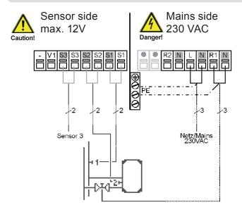
**Low voltage** max. 12VAC/DC connection in the left-hand terminal compartment!
