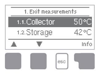
The menu "1. Measurement values" serves to display the currently measured temperatures.
