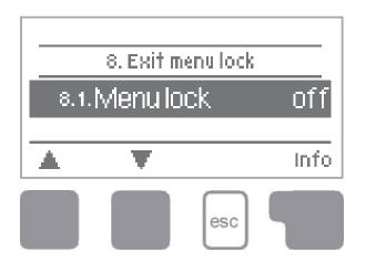
Menu "8. Menu lock" can be used to secure the controller against unintentional changing of the set values.
