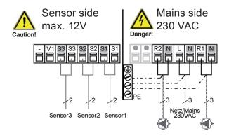
Brief description of switching function: The  $\Delta T$  function sensor 1 > sensor 2 switches the pump to relay R.
