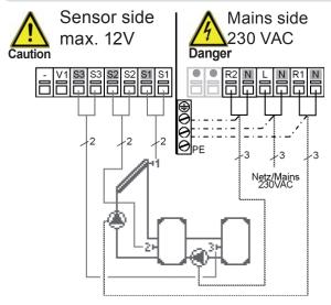
**Low voltage** max. 12VAC/DC connection in the left-hand terminal compartment!
