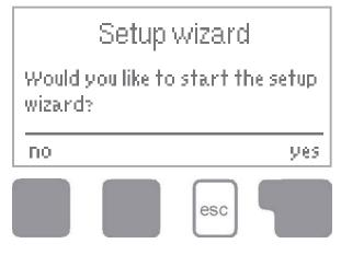
The first time the controller is turned on and after the language and time are set, a query appears as to whether you want to parametrise the controller using the commissioning help or not. The commissioning help can also be terminated or called up again at any time in the special functions menu. The commissioning help guides you through the necessary basic settings in the correct order, and provides
