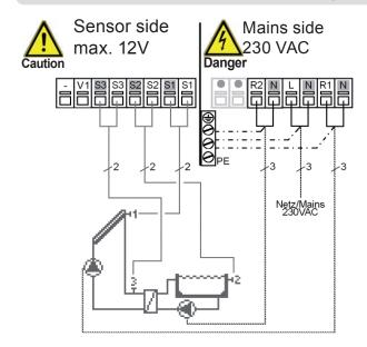
**Low voltage** max. 12VAC/DC connection in the left-hand terminal compartment!
