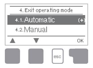
In menu "4. Operating modes" the controller can either be placed in automatic mode, switched off, or placed in a manual operating mode.
