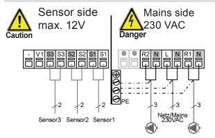
**Low voltage** max. 12VAC/DC connection in the left-hand terminal compartment!
