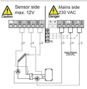
**Low voltage** max. 12VAC/DC connection in the left-hand terminal compartment!
