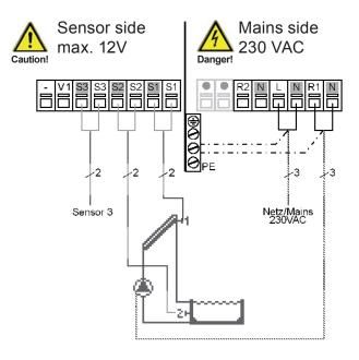
**Low voltage** max. 12VAC/DC connection in the left-hand terminal compartment!
