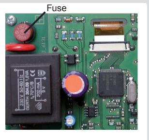
If the mains voltage is switched on and the controller still does not function or display anything, then the internal device fuse may be defective. In that case, open the device as described under C, remove the old fuse and check it.
