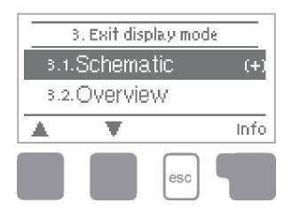
Menu "3. Display mode" is used to define the controller's display for normal operation.
