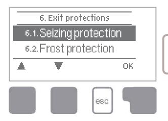
Menu "6. Protective functions" can be used to activate and set various protective functions.
