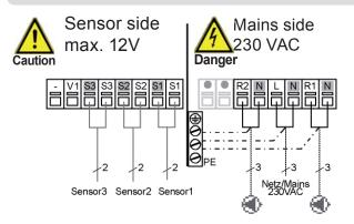
Brief description of switching function: The  $\Delta T$  function sensor 1 > sensor 2 switches the pump to relay R1. The  $\Delta T$  function 2 > sensor 3 switches the pump to relay R2.
