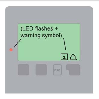
If the controller detects a malfunction, the red light flashes and the warning symbol also appears in the display. If the error is no longer present, the warning symbol changes to an info symbol and the red light no longer flashes.
