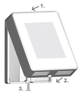
Refit the base and fasten with screw. Switch on mains voltage and place °CALEON in operation.
