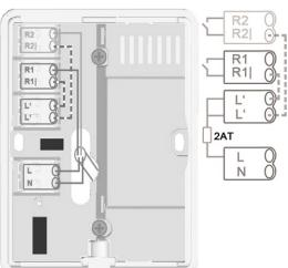
Unscrew the screw, remove the cable cover and connect the electric as described.
