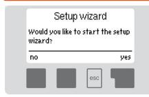
The setup wizard will rapidly guide you through the settings which need to be performed in a logically reasonable sequence. This way, any misadjustment is avoided and the parametrising is simplified.
