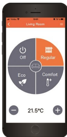
Select operating mode and set tar- get room temperature
