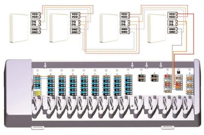
**Example 2:** Tree structure. Several stub lines lead from one main line to the individual sensors.
