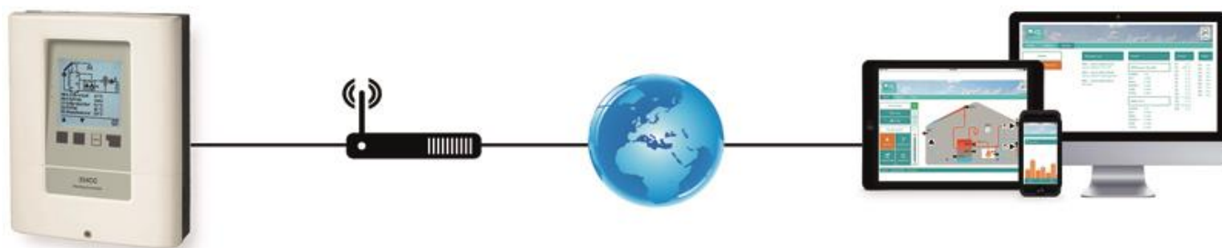
Application example: XHCC with direct Ethernet connection
