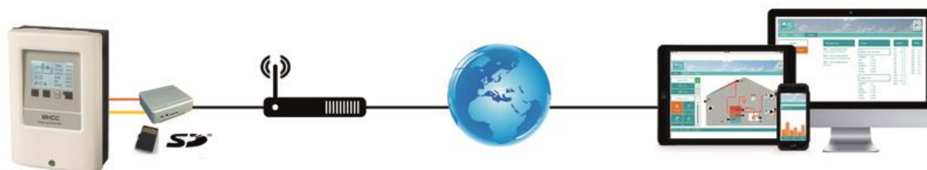
Application example: MHCC with Ethernet connection via data logger
