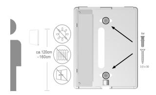
Mount the sensor in a suitable location.
