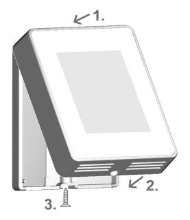
Refit the base and fasten with screw. Switch on mains voltage and place  ${}^{\circ}\text{CALEON}$  in operation.
